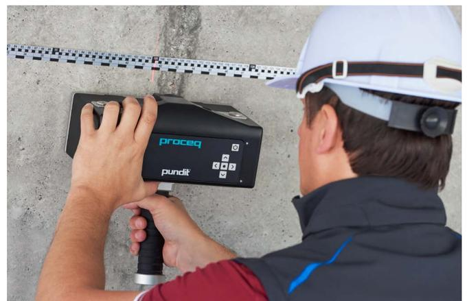
Error-free positioning with the Pundit Live tape measure
