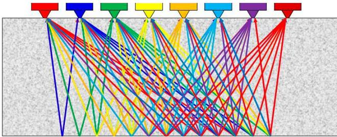
8 channel pulse echo measuring head principle
