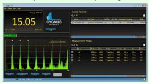
Once the survey results are in CygLink there is a range of different ways to view the data. This includes; linear, grid, colour 2D and 3D representations. The data can be exported to a spreadsheet program e.g. Excel.
