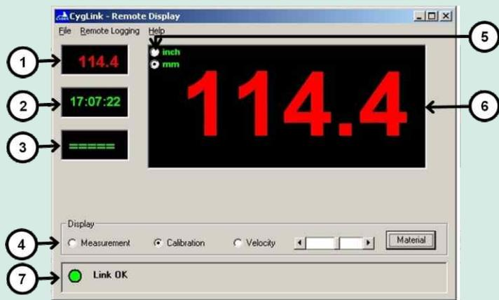
1. Displays the last thickness measurement value
