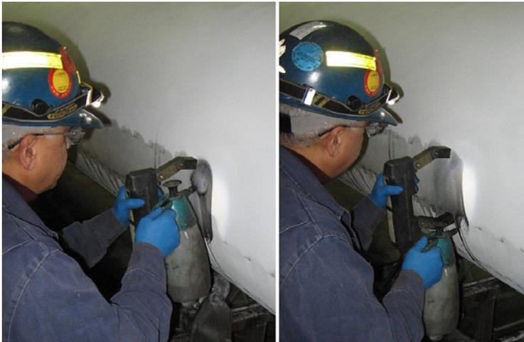
Wet MT is, obviously, messy, and requires surface preparation and post-inspection cleaning before being able to repaint or recoat the weld, which is time consuming. Other shortcomings of this inspection method are its inability to measure the depth of defects and its lack of archiving capabilities.
