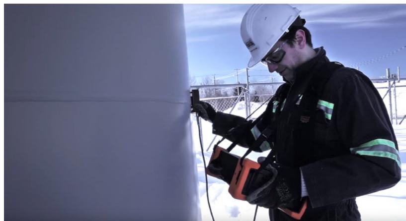
The **Sharck** is also designed to scan at speeds up to 200 mm/s (8 in/s), record inspection data fully, and display it as intuitive 2D/3D C-scans thanks to the **Ectane® 2** and **Magnifi®**. Performing the inspection with the new **Reddy™** (unavailable at the time) could have offered more portability and flexibility.
