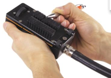
Unlike wet MT, the innovative tangential ECA (TECA™) technology incorporated into the **Sharck** probe can size the length and depth of cracks. It can do this without surface preparation of any kind, as it is designed to monitor liftoff (as opposed to cancelling it out) and compensate for it.
