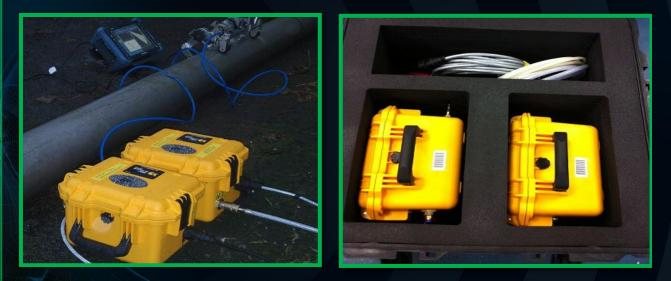
The system is available in both medium or high volume output and due to the utilisation of the uniquely designed Compact Self Priming Diaphragm Pump, we are able to accommodate a broad spectrum of use, from standard single probe inspection, to double sided simultaneous Phased Array and TofD inspections. An additional feature for both systems is the variable flow control and both are equipped with a 15 metre, 8mm diameter hose.
