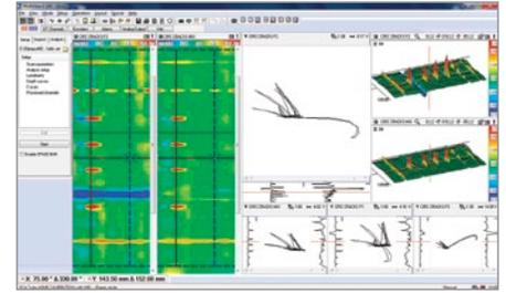
Example of MS5800 with 4x 32-channel ECA probes connected through 2 ECA multiplexers.
