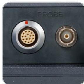
The 16-way LEMO connector also supports the PowerLink NORTEC technology, which features automatic probe recognition and instrument presets for quicker setups.
