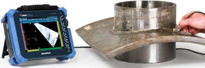
The OmniScan PA is at the heart of the manual and semiautomated phased array weld inspection solutions developed by Olympus for the oil and gas industry. These systems can be used for inspection in compliance with ASME, API, and other code criteria, while offering high-speed detection capabilities, and facilitating indication interpretation.
