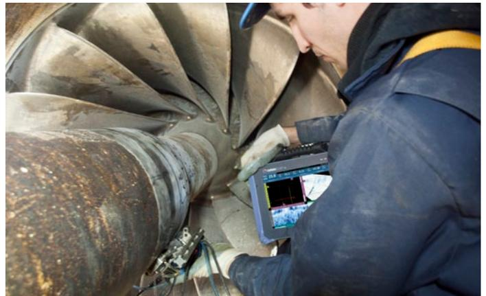
Using ultrasonic techniques, inspection of components can detect cracks, wall loss, and other damage. With the capacity for both angle and linear zero-degree beams, the OmniScan SX is a very cost-efficient solution for this type of single-group inspection.
