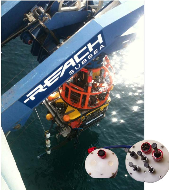
The Orion sensor array only needs to be brought in the approximate vicinity of the utility line to calculate a relative position. Using at least two 3D magnetic field sensors, a triaxial accelerometer and digital compass, Orion identifies the horizontal offset, vertical depth, tone current strength and yaw
