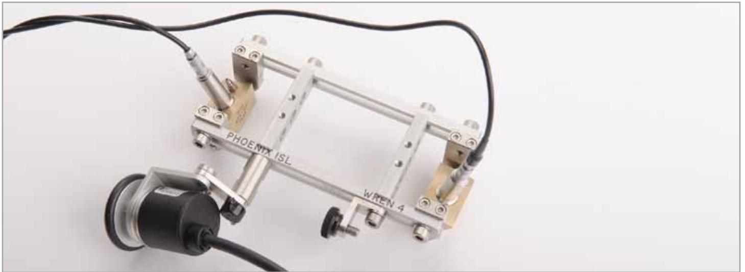
WREN 4 - Weld Root Erosion Scanner
