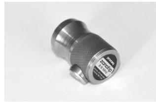
The 2.5 MHz **single-element** transducer is more compact, requires only one cable and is therefore more suited for measuring in confined spaces.
