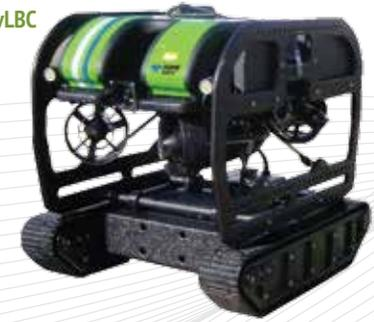
Speed: vLBC - Up to 35 m/min (115 ft/min)
