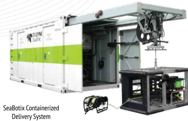
The CDS can be installed on any vessel of opportunity via a single point lifting system and can be operated by two persons from vessels as small as 40 m (131 ft). It is simple to deploy, operate and service. The CDS can handle deep water missions with a variety of sensors such as sonar, NDT, tracking, high resolution cameras and grabbers.
