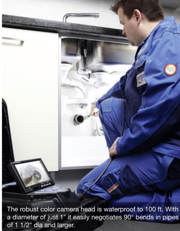
The robust color camera head is waterproof to 100 ft. With a diameter of just 1" it easily negotiates 90° bends in pipes of 1 1/2" dia and larger.
