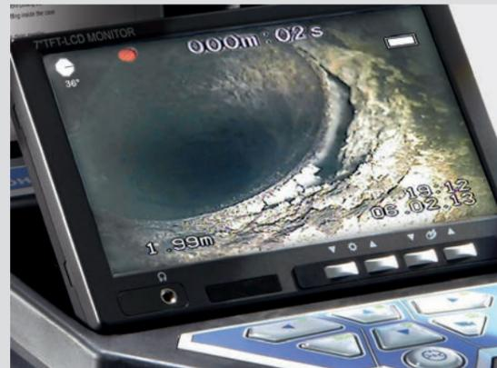
The "Save function" (Wohler VIS 250) makes it possible to save and view what you see at the push of a button. The integrated position indicator (Wohler VIS 250) ensures you keep your sense of orientation in the pipe.
